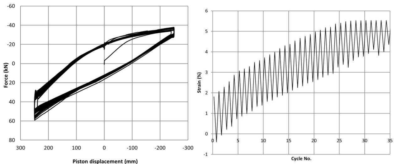
**Figure 3:** Force displacement diagram (left); hoop strain with respect of the number of cycles (right).
