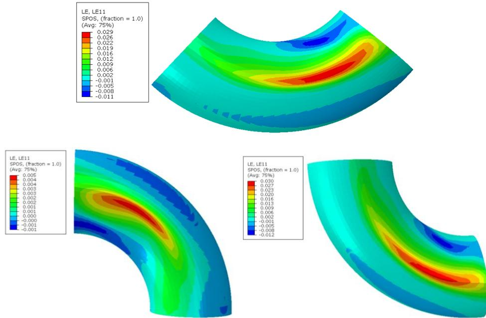
**Figure 6:** Distribution of hoop strain for Elbow1 (Up) Elbow2 (left), Elbow 3 (right).
