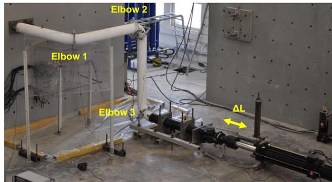
**Figure 1:** Experimental set up for the 8-inch-diameter piping system.
