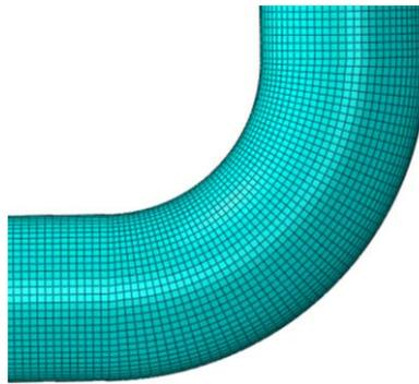
**Figure 5:** Elbow meshing detail.
