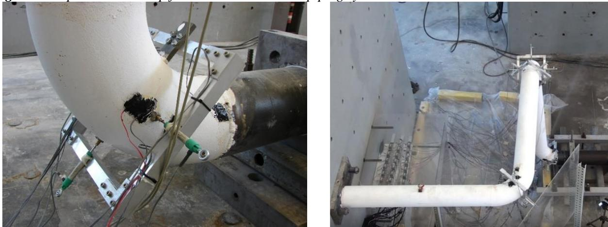
**Figure 2:** Experimental instrumentation (left); failure at Elbow 3 (right).
